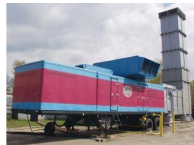
Mobile power station
