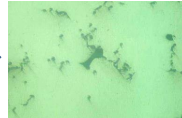
Shrinkage and microporosity in the material
