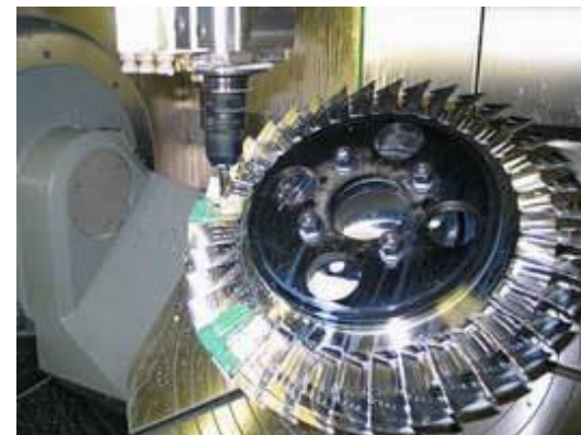
High-speed milling of mono-wheels
